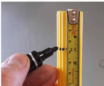
**3.** Slide the connector over the cut end of the stringer upto the pen mark and drill a 6mm hole through the stringer using the drilled holes in the connector as a guide.
