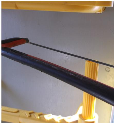
**1.** Install the first length of stringer through the steps as detailed in the integrated ladder fitting instructions. Cut the end of the installed stringer approximately equidistant between two rungs, ensure the cut is square. Any single length of stringer must be supported by at least 2 rungs.
